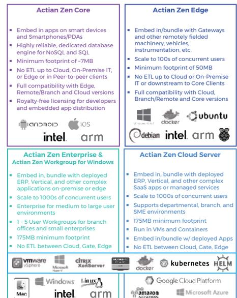
The Actian Zen database family is built with a single, modular architecture that scales from a core set of libraries capable of single-user client data management to a fullfledged, enterprise-grade server, capable of supporting thousands of users on multicore, VM cloud environments (Nutanix AHV, VMware vSphere, Microsoft HyperV, and Citrix XenServer) or in Docker
